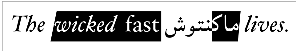
Figure 10-19 Discontiguous highlighting from offsets 4 to 19 in mixed-direction text
