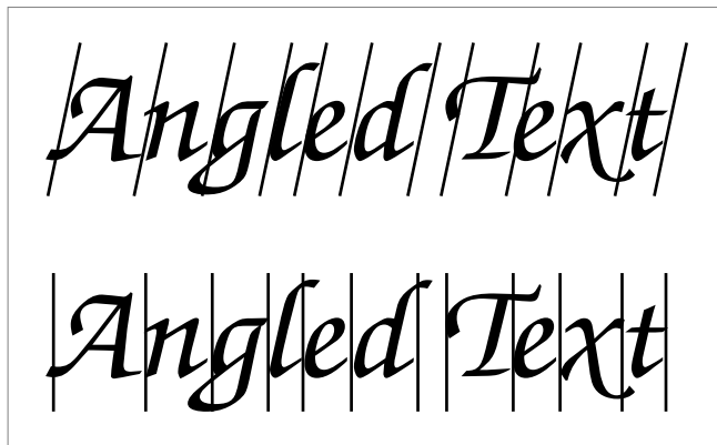
Figure 10-15 Drawing all possible caret positions in a layout shape's text
